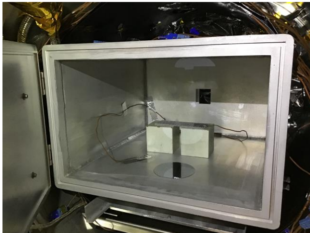
Resin-coated foam inside effusion cell
