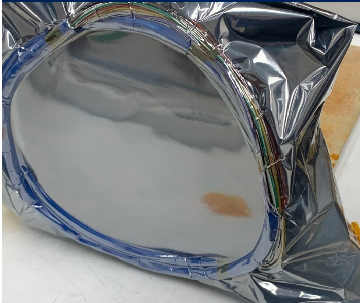
Co60 fixture with sample wire bag sealed
