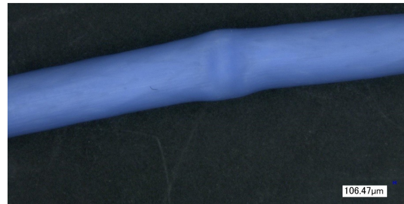
Bent wire outer insulation "crumpled" but did not fail 20x mag
