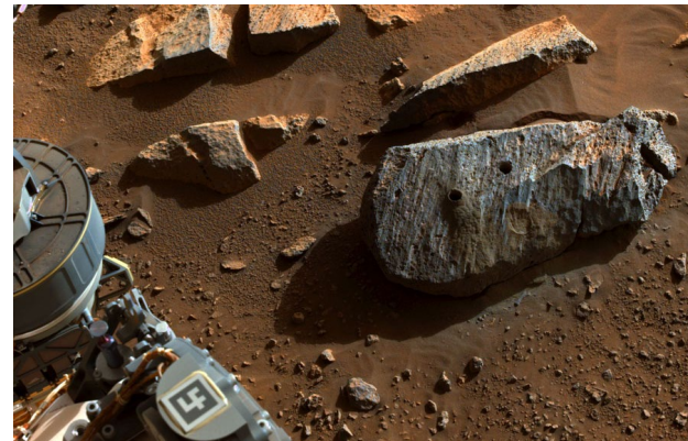
Image: NASA's Perseverance rover on Sept. 7, 2021, PDT (Sept. 8, EDT), shows two holes where the rover's drill obtained chalk stick-sized samples from rock nicknamed "Rochette." Credit: NASA/JPL-Caltech
