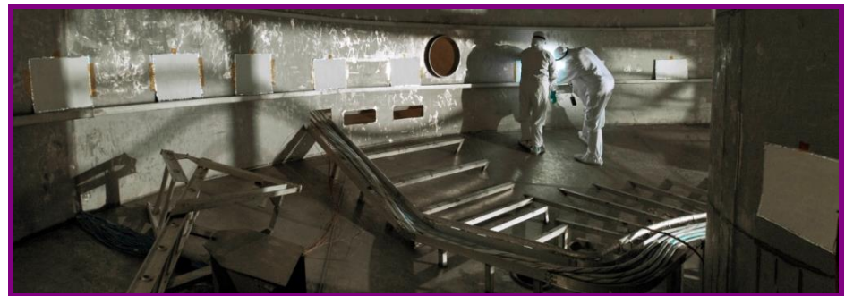
As shown, NASA GSFC installed MAC samples on the walls of the plenum in the Chamber A test facility prior to the start of the tests
