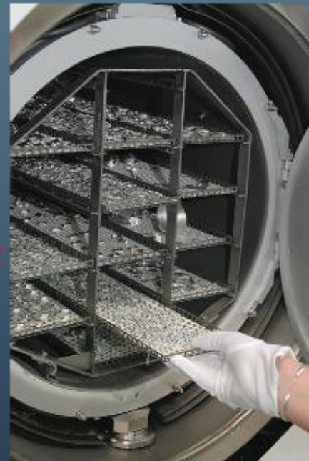
Coating Silver with Aluminum Oxide http://www.glassanweb.com/
