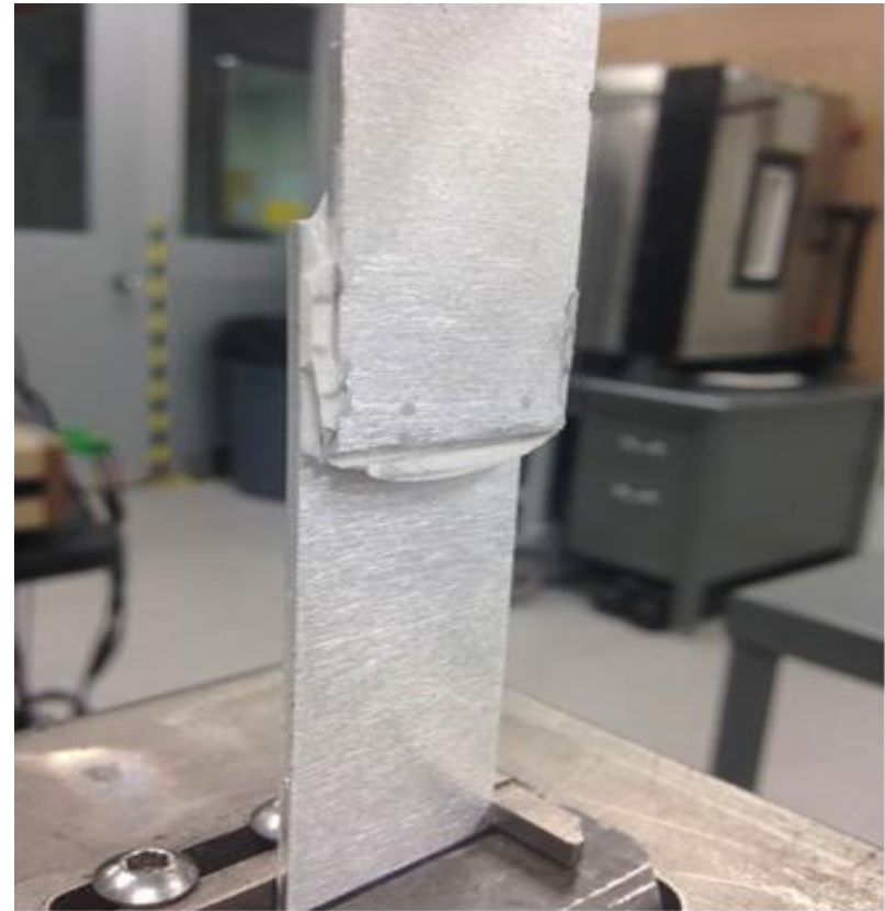
Right: Typical adhesive lap shear sample loaded into test apparatus
