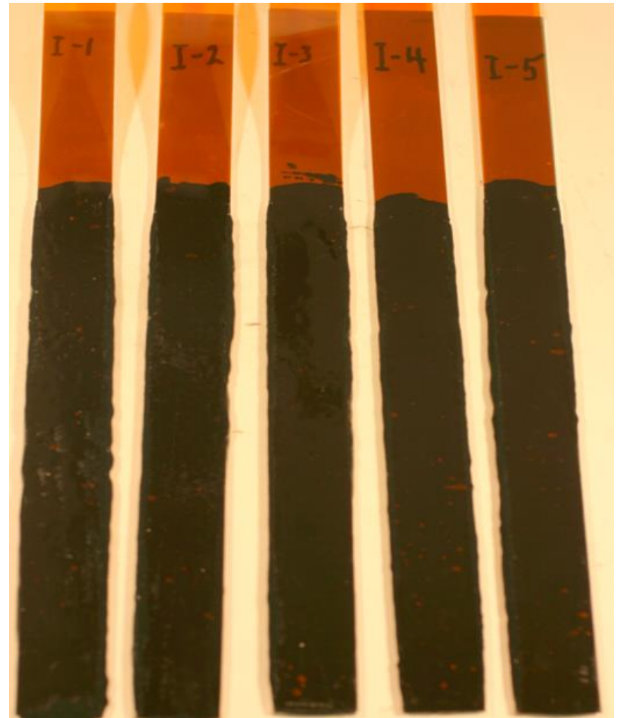
Peel test samples (Stycast 2850FT)
