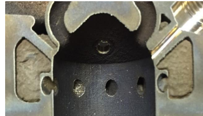
Remnant Powder Permanently Trapped in Interior Cavities following Inadequate Cleaning & Post Thermal Processing
