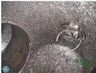
Burrs Trapped in Machined Hole
