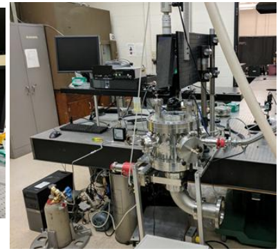
FLSP environmental chamber
